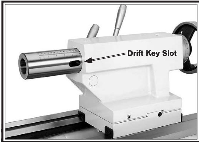
Figure 49. Drift key slot in the side of the quill.
